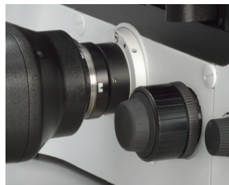
Imaging port with large 25 field number
