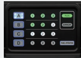
Signaled by white light for properly set cassettes, blinked white light for not properly set cassettes, green light for the completion of scanning.
