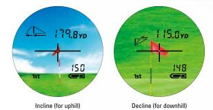
The upper figure shows the "slope adjusted distance" and the lower figure is the "actual distance". Both are displayed simultaneously in the internal display.
