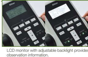
The brightness of the LCD monitor and LED indicators is adjustable
